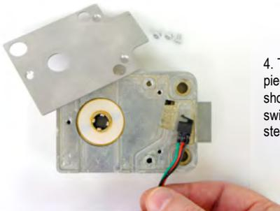
4. The switch comes with a very small piece of foam attached to the front, as shown here. The foam helps hold the switch in the lock cavity when the steel cover plate is attached.
