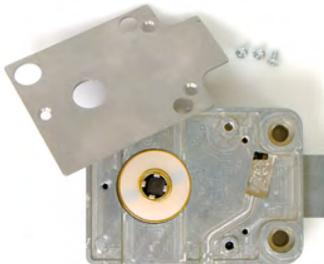
2. Let the lock case lie on its cover side when removing the steel plate to make sure the drive cam and white plastic washer stay in place.
