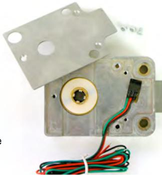
5. With the switch in place in the lock body cavity, route the three wires in the recessed channel. Make sure all three wires are completely within the channel so they will not be pinched or crushed when the steel plate is re-installed.
