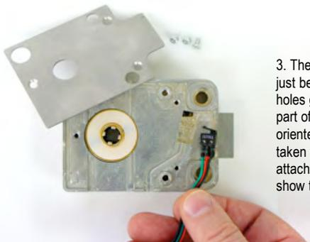
3. The pre-wired switch has two holes just below the small lever arm. These holes go over two small posts cast as part of the lock body, with the lever arm oriented as shown. This photograph was taken without the small foam pad attached to the front of the switch to show the two small holes.
